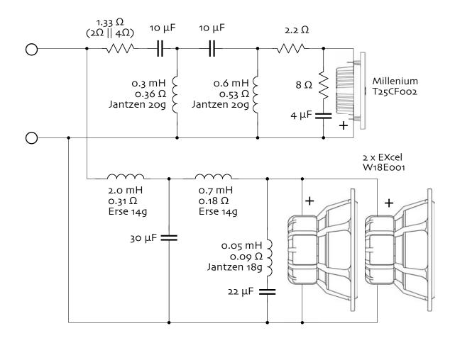
SEAS MTM Crossover drivers as used in Thor/Odin Note: bafflestep for 10" baffle width (a full 6 dB is implemented) see <http://www.htguide.com/forum/showthread.php4?t=26754> for more info designed by jimangie1973 drawn by dld / 04-september-2007
